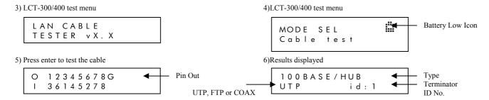
7)Use MODE/SEL to toggle between cable pin out screen and result display, press ESC back to test menu.
