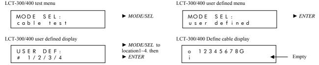
Use the **ENTER** key to set digits 1-8, G or blank (not connected), then press **MODE/SEL** to move to the next space. When complete press ESC (step no. 5 to 6).
