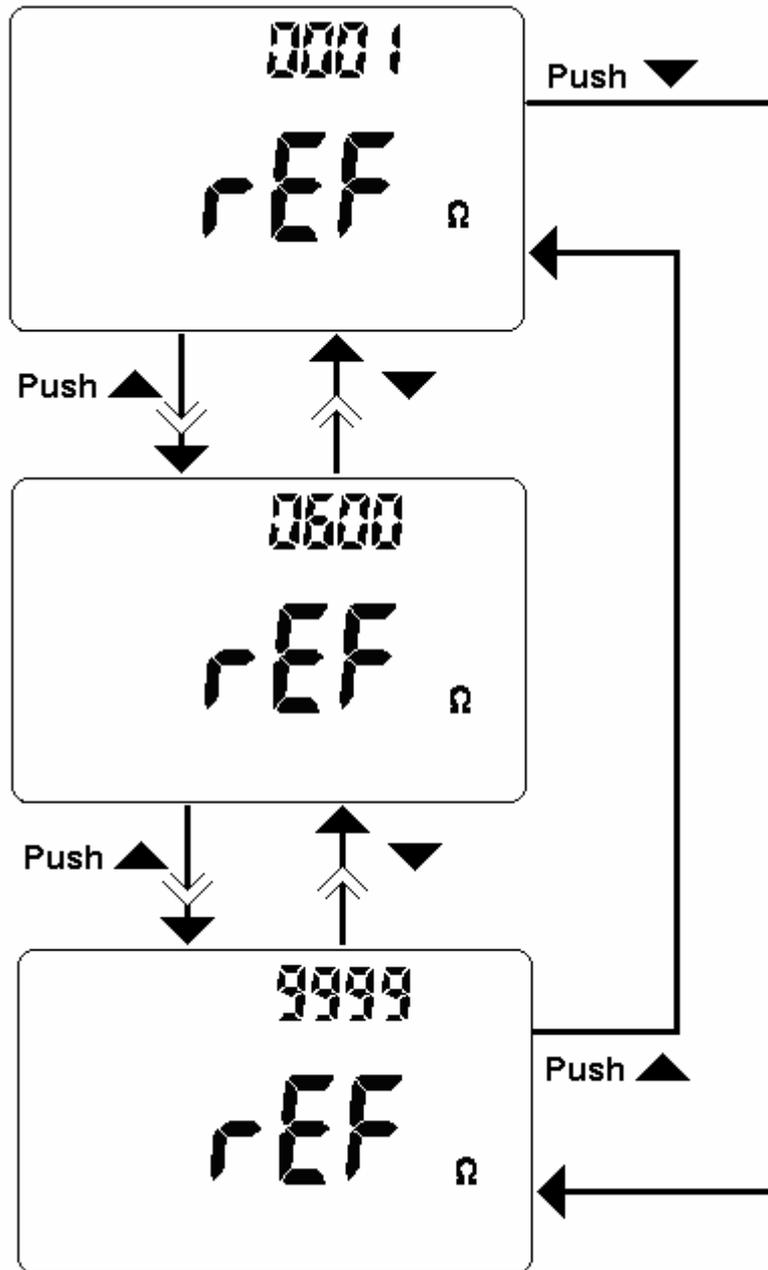
Figure- 21 Reference Impedance for dBm
