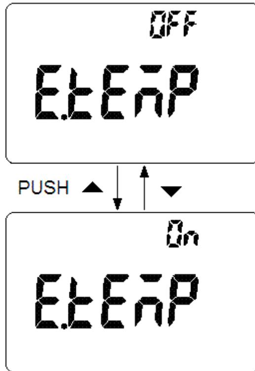
**Figure- 16 Enable Environment Temperature display**
