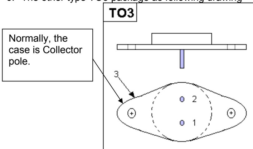
Figure- 56 TO-3 Transistor
