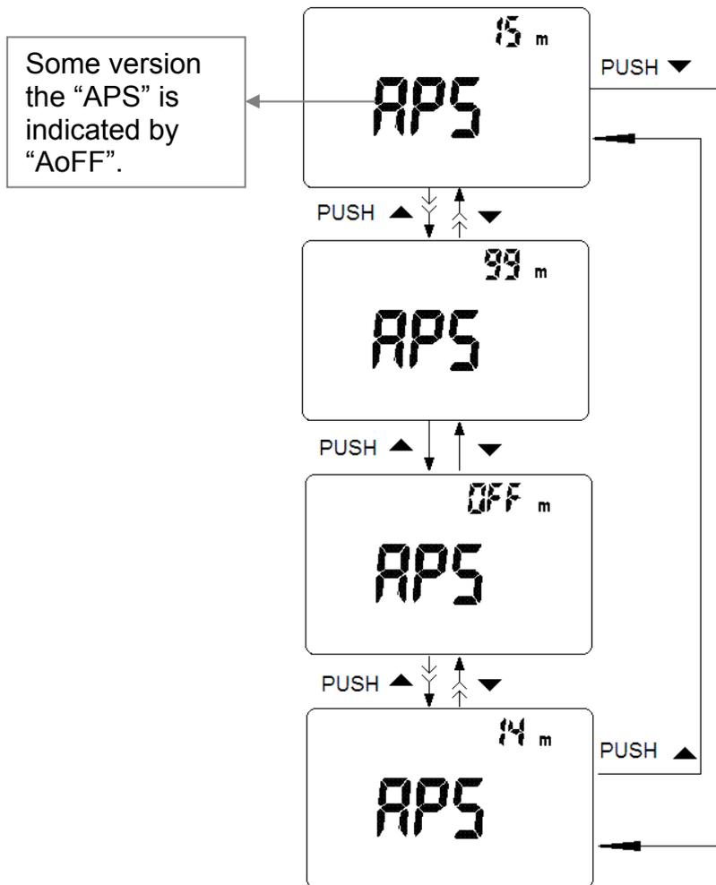
Figure- 17 Auto power saving setup
