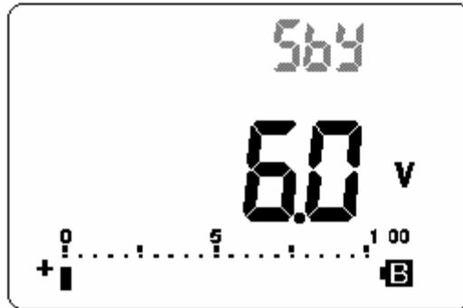
Figure- 63 Battery capacity display as trickle
