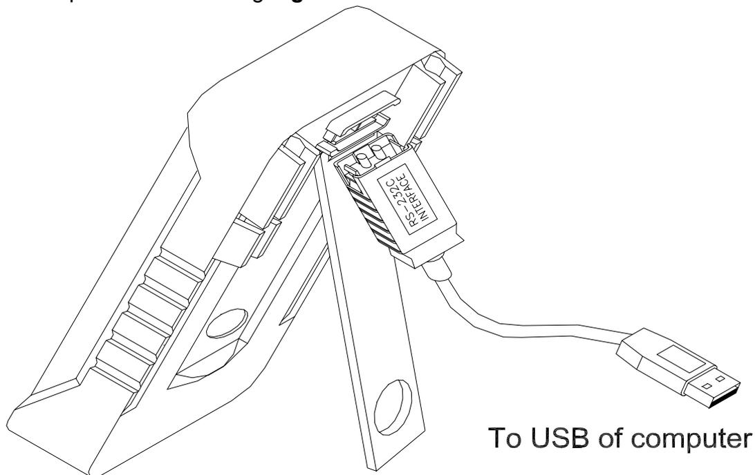
**Figure- 37 Cable Connection for Communication**
