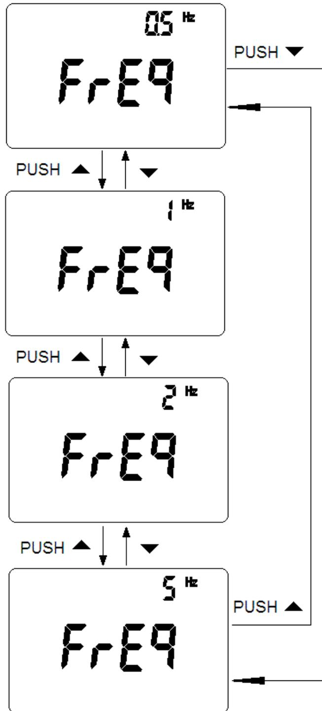
Figure- 12 Minimum Frequency Setup
