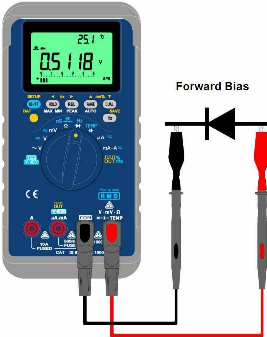
Figure- 52 Forward Bias of Diode Measurement
