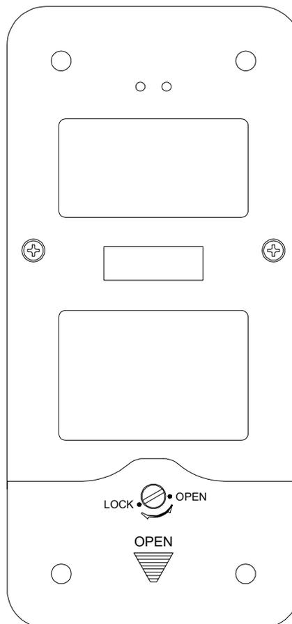
2. Turn the screw on the battery cover from LOCK to OPEN position by counterclockwise.
