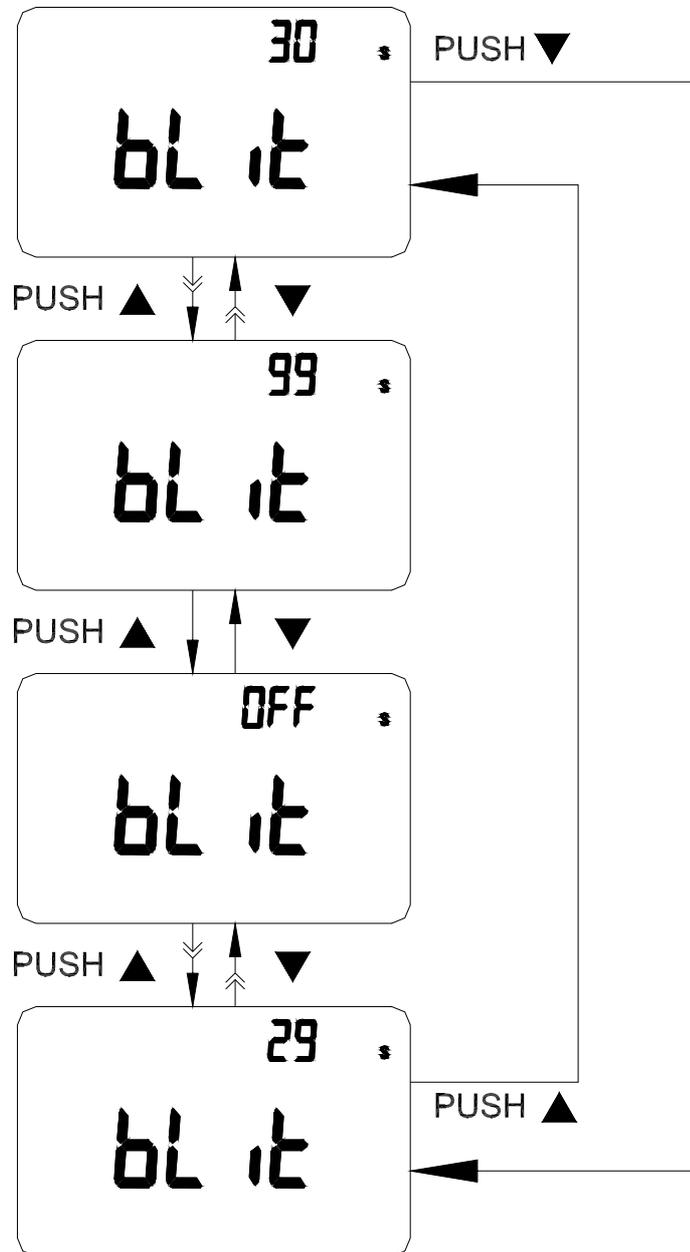
Figure- 18 Backlit Timer Setup
