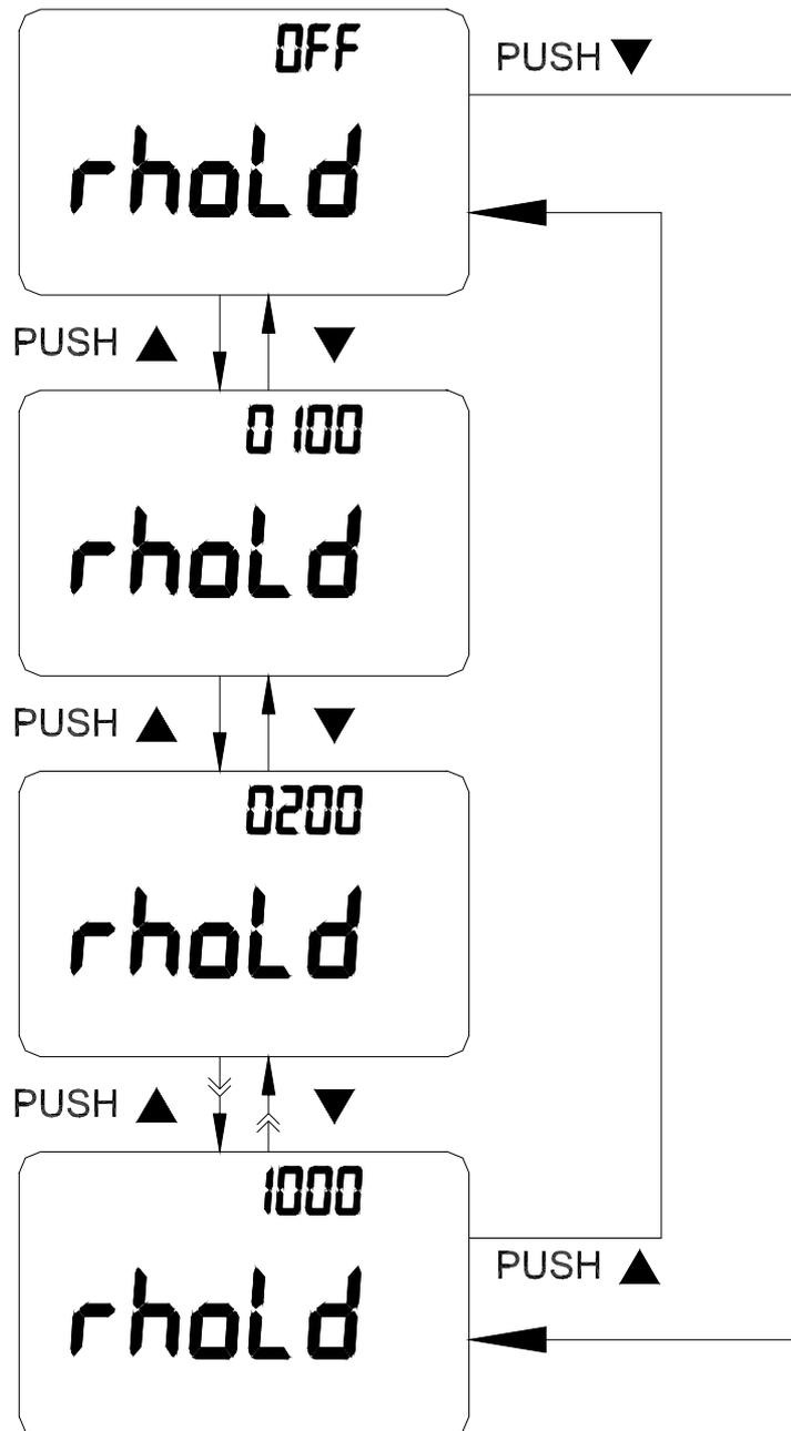
Figure- 15 Data Hold/ Refresh Hold Setup
