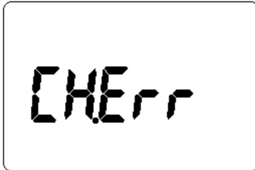
**Figure- 27 Charge Terminal Alert**
