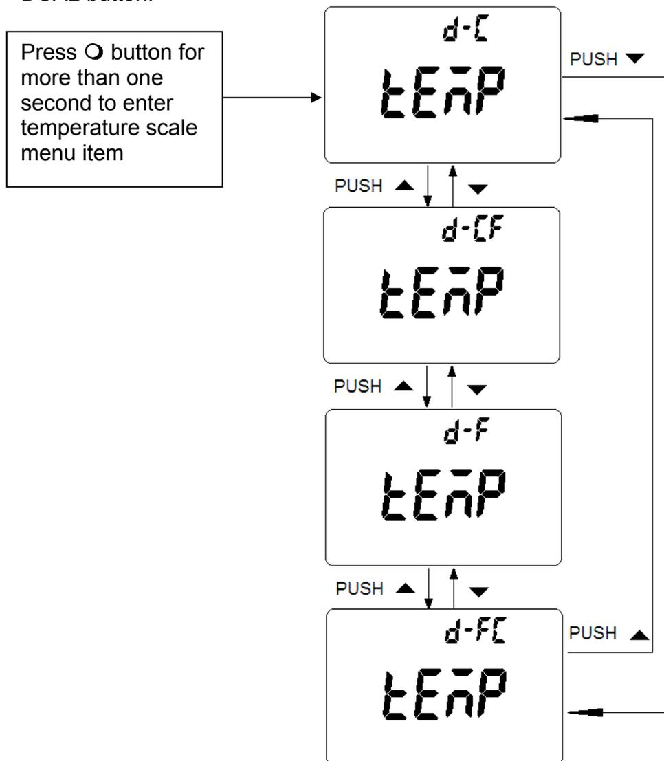
Figure- 14 Temperature Unit Setup
