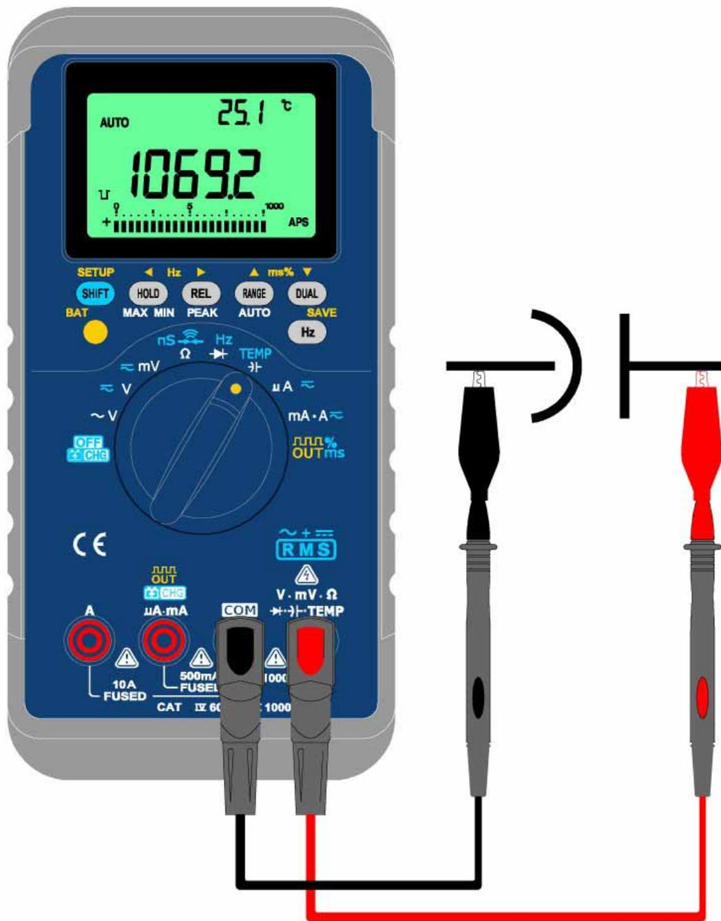
Figure- 54 Capacitance measurement
