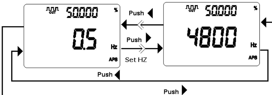
Figure- 23 Frequency Adjustment for Square wave
