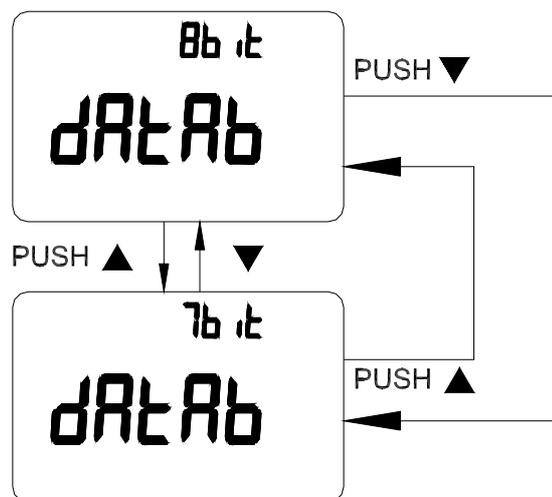
Figure- 8 Data bit setup for remote control
