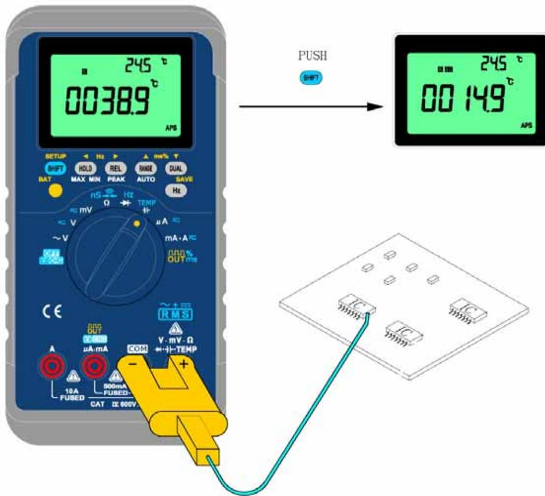
Figure- 60 Surface temperature measurement
