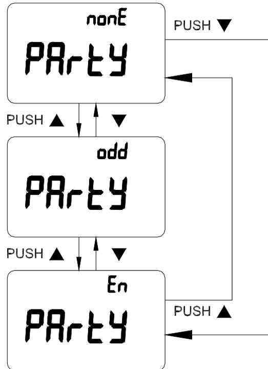
Figure- 7 Parity Check setup for remote control
