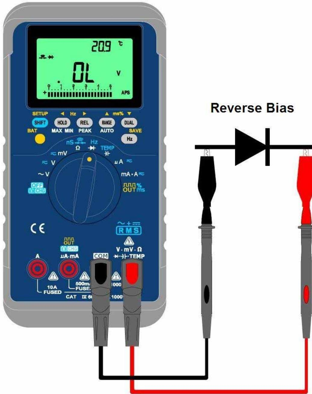
Figure- 53 Reverse Bias of Diode Measurement
