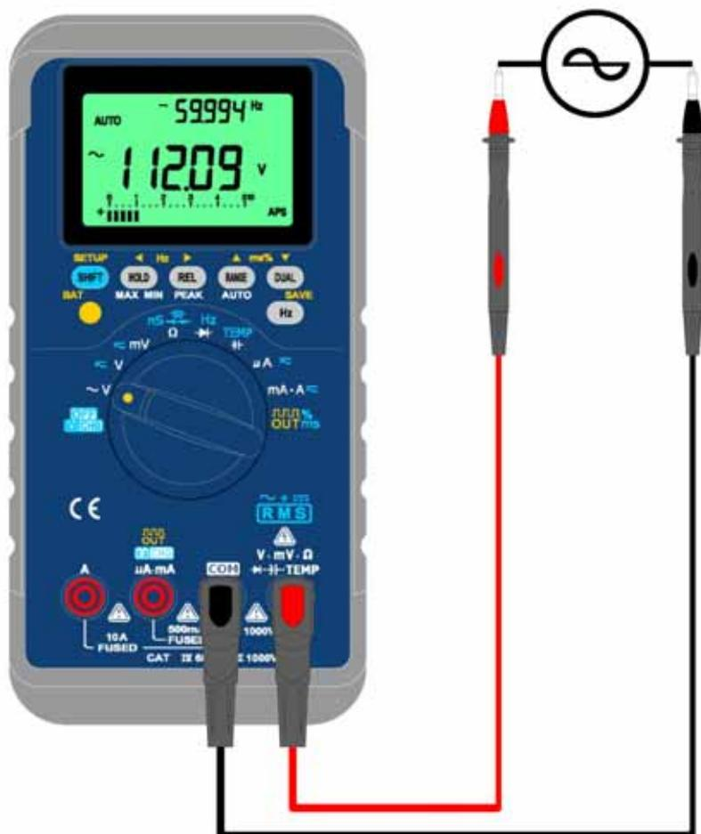
Figure- 42 Line power Voltage measurement
