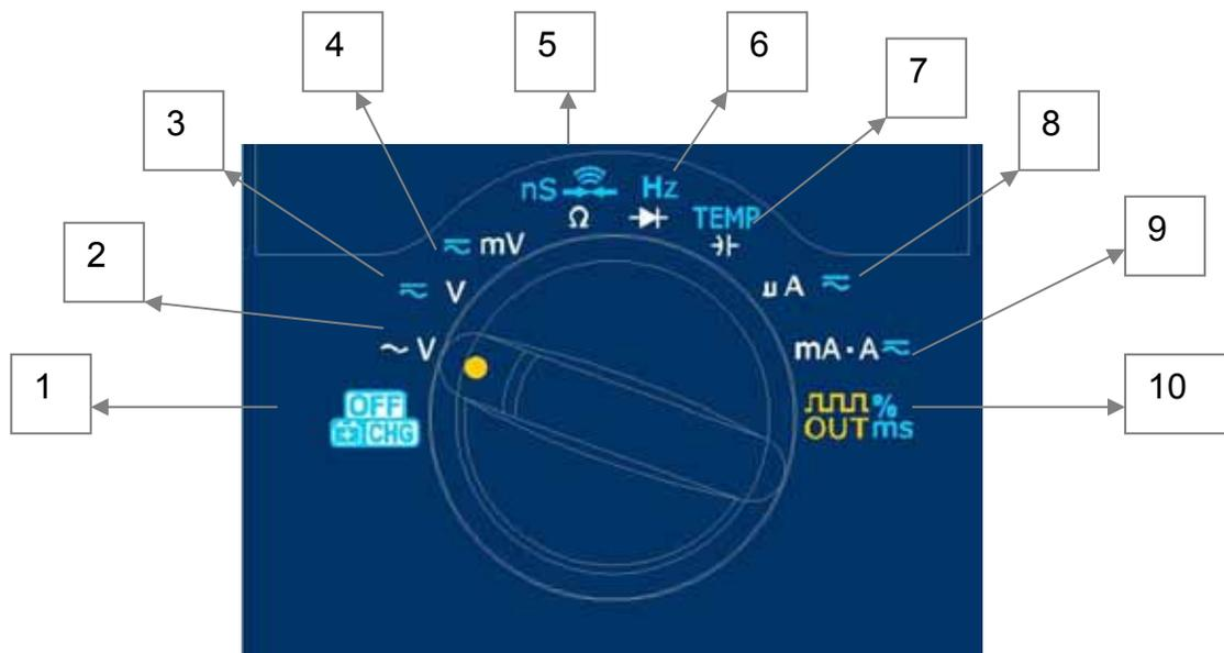
Figure- 3 Rotary Switch for selecting function
