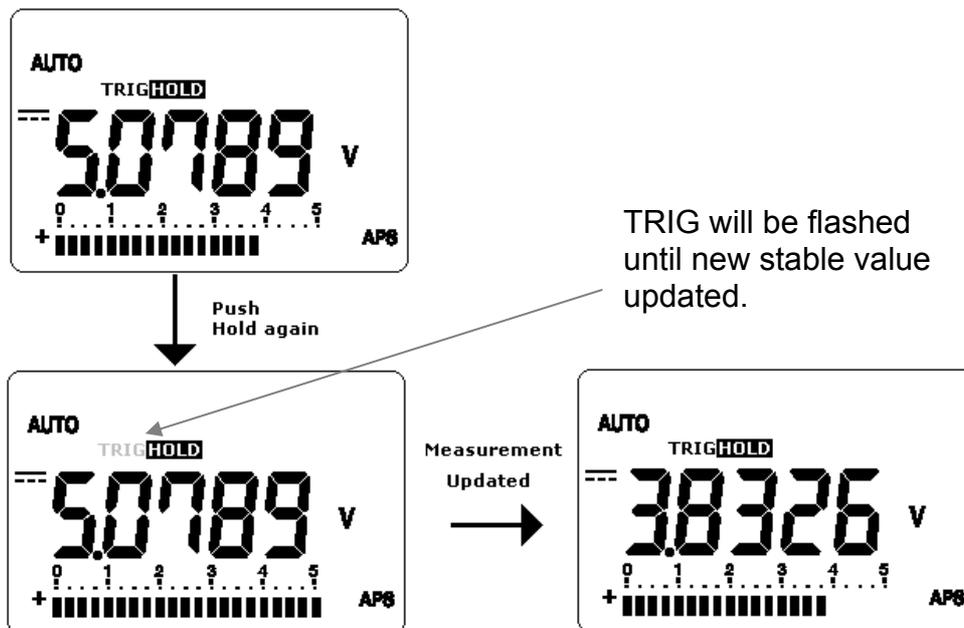
Figure- 31 Trigger Hold
