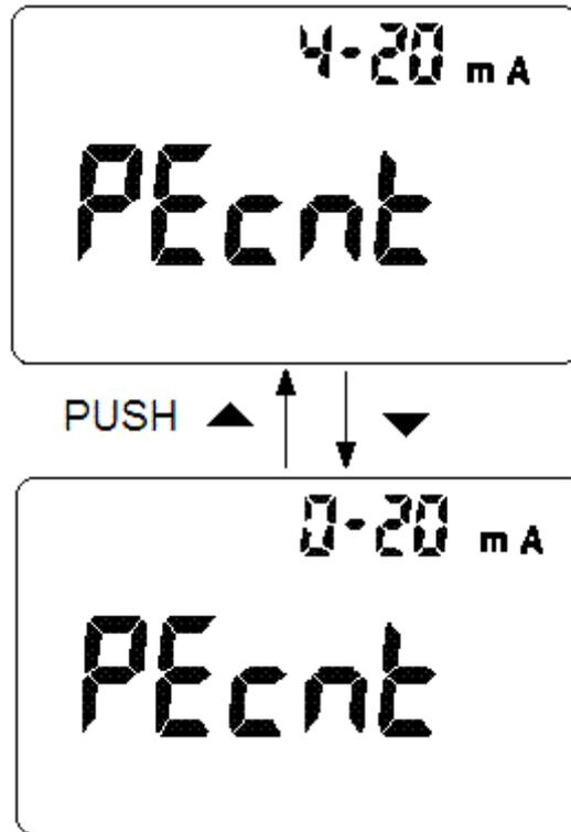
**Figure- 11 The % scale Setup for mA measuring**
