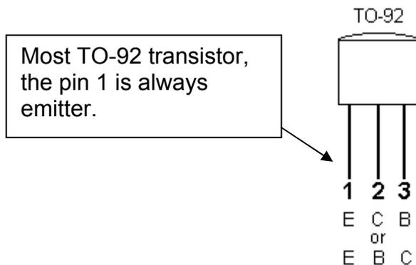
**Figure- 55 TO-92 Transistor**
