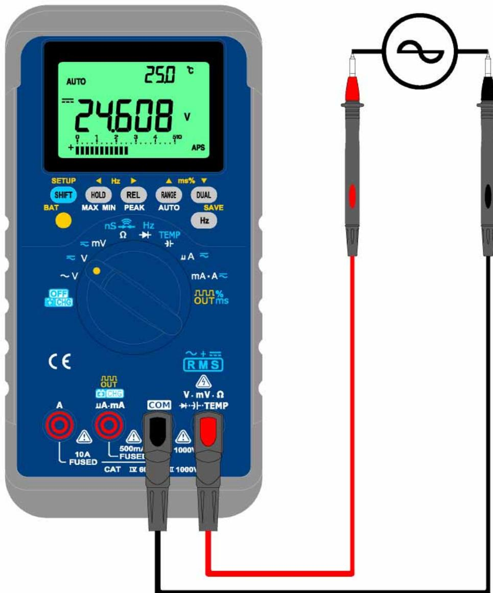
Figure- 43 Check the power source of transmitter
