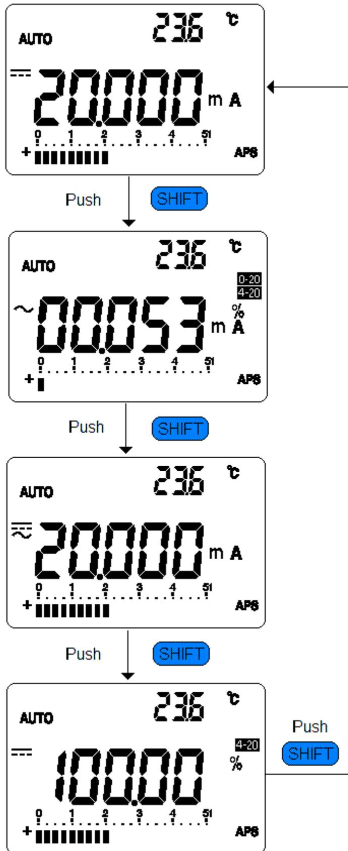
Figure- 41 Shift mA function by Blue button
