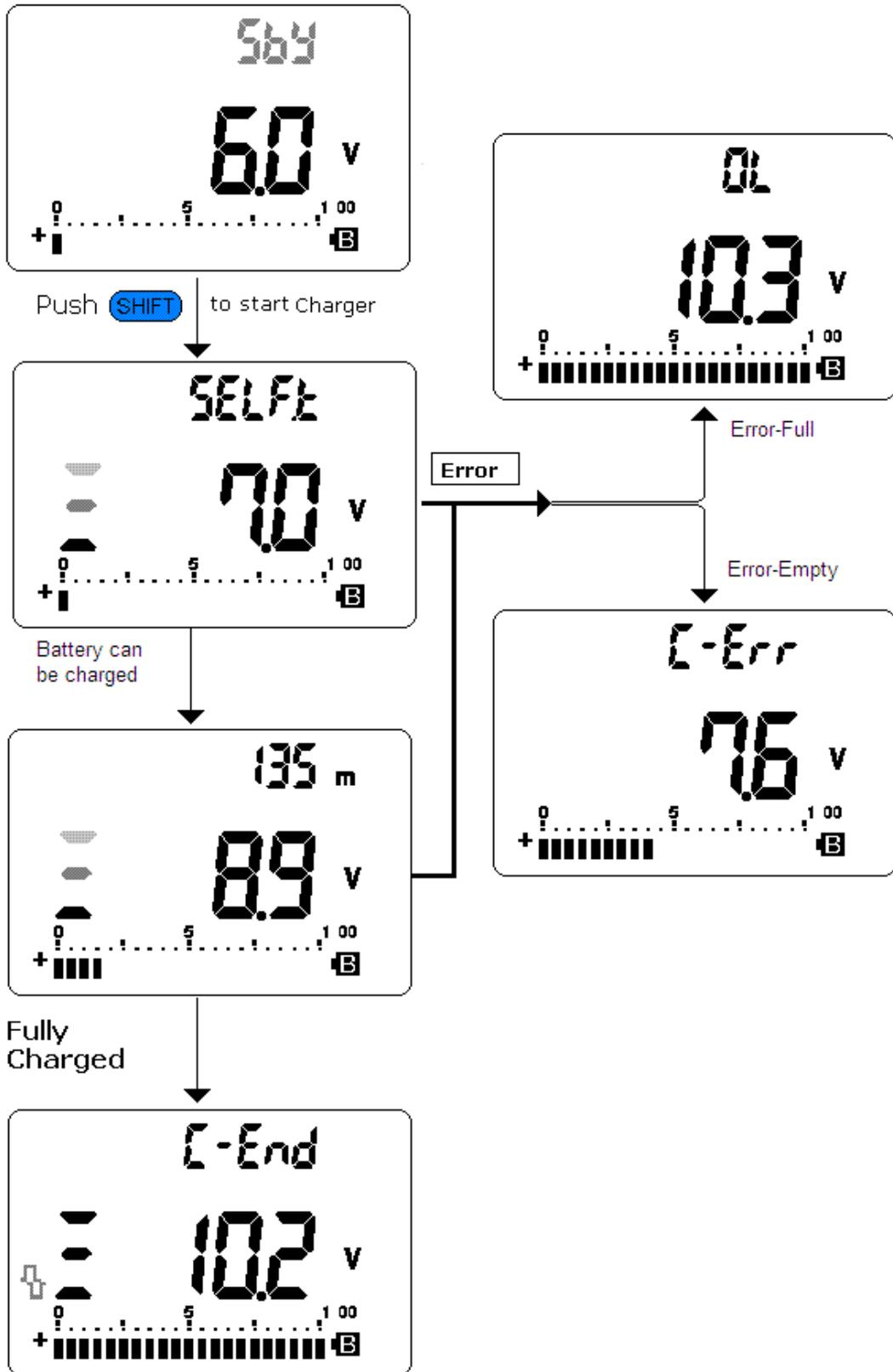
Figure- 68 Battery charging procedures
