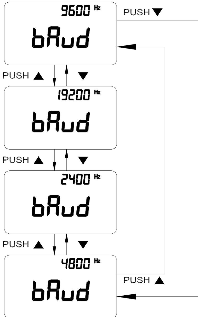
**Figure- 6 Baud rate setup for remote control**
