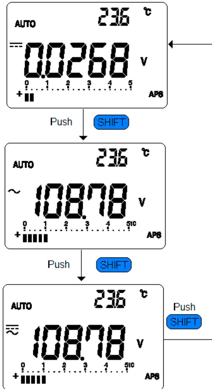
Figure- 40 Shift V function by Blue button
