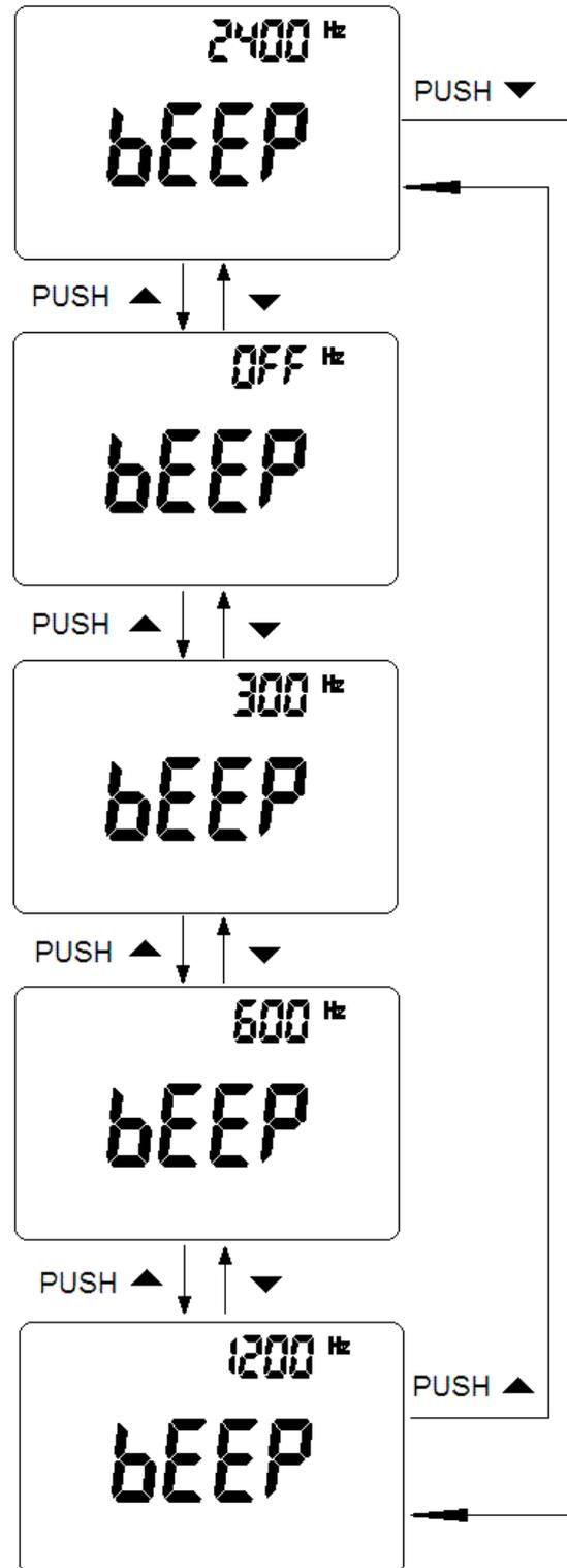
**Figure- 13 Driving frequency of Beeper setup**
