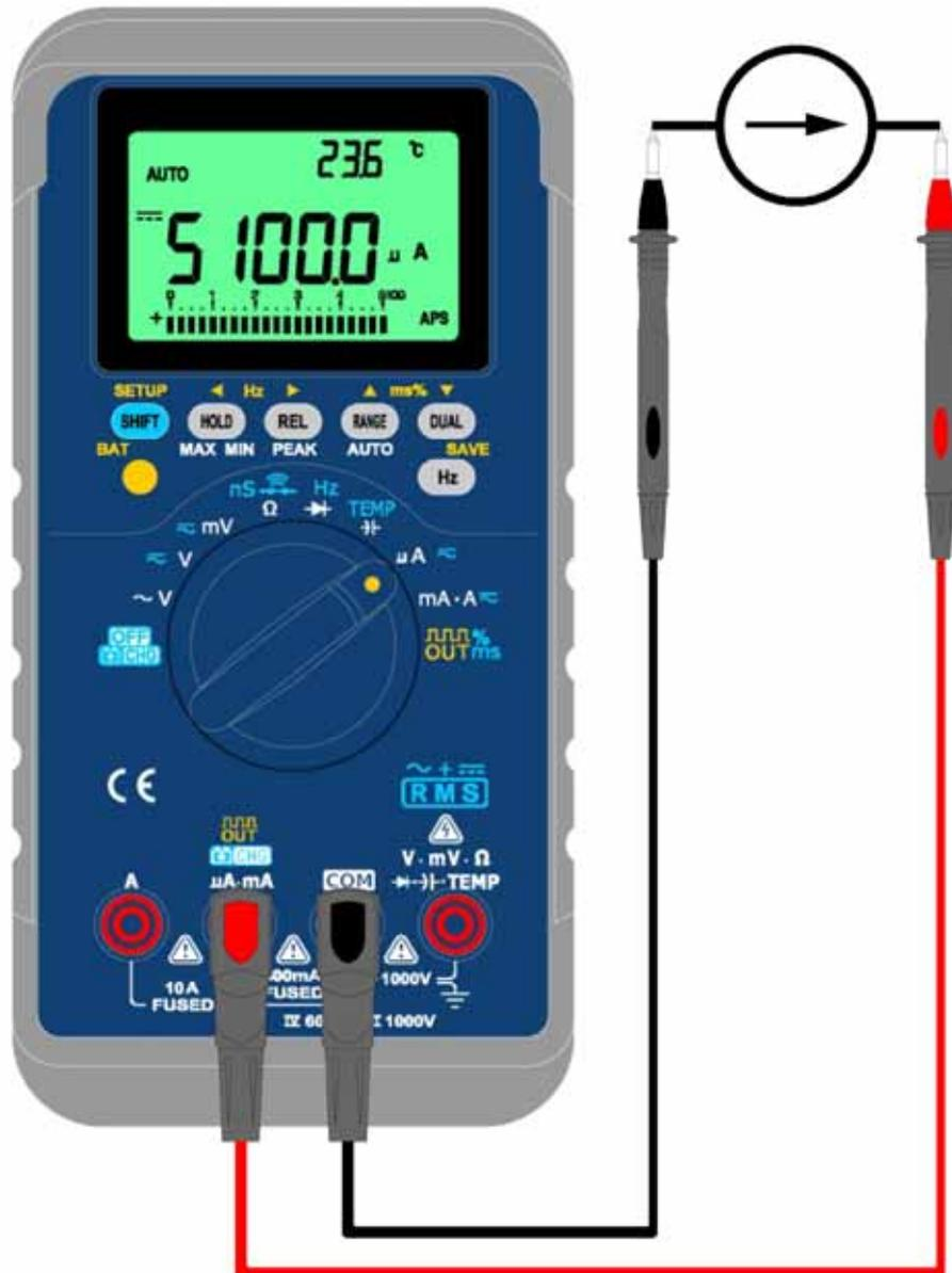
Figure- 44  $\mu\text{A}$  Measurement
