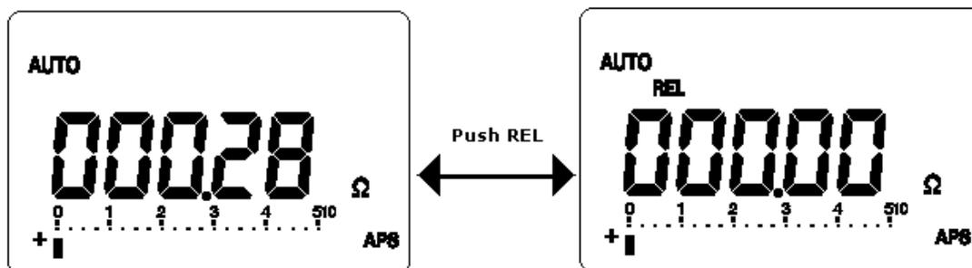
**Figure- 33 Relative (Zero) Operation**
