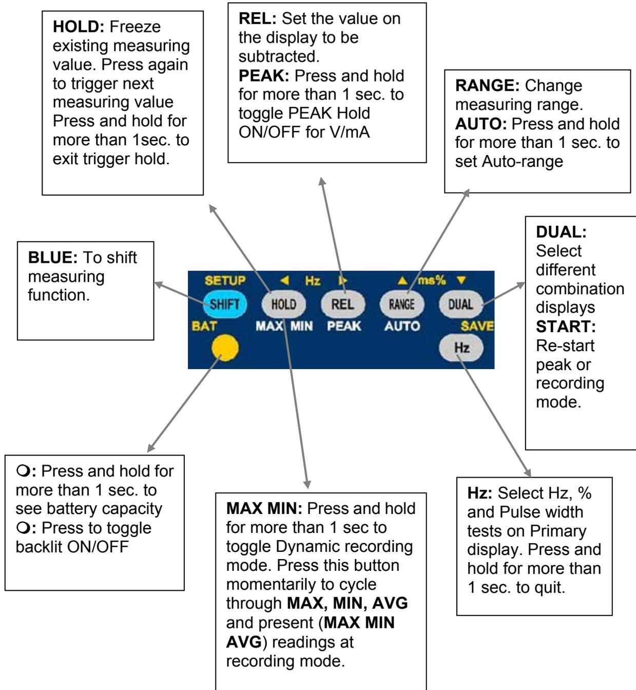
Figure- 5 Pushbuttons
