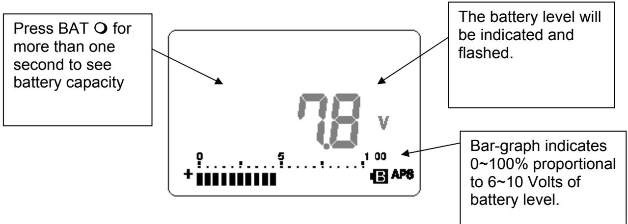
**Figure- 28 Capacity check of battery**
