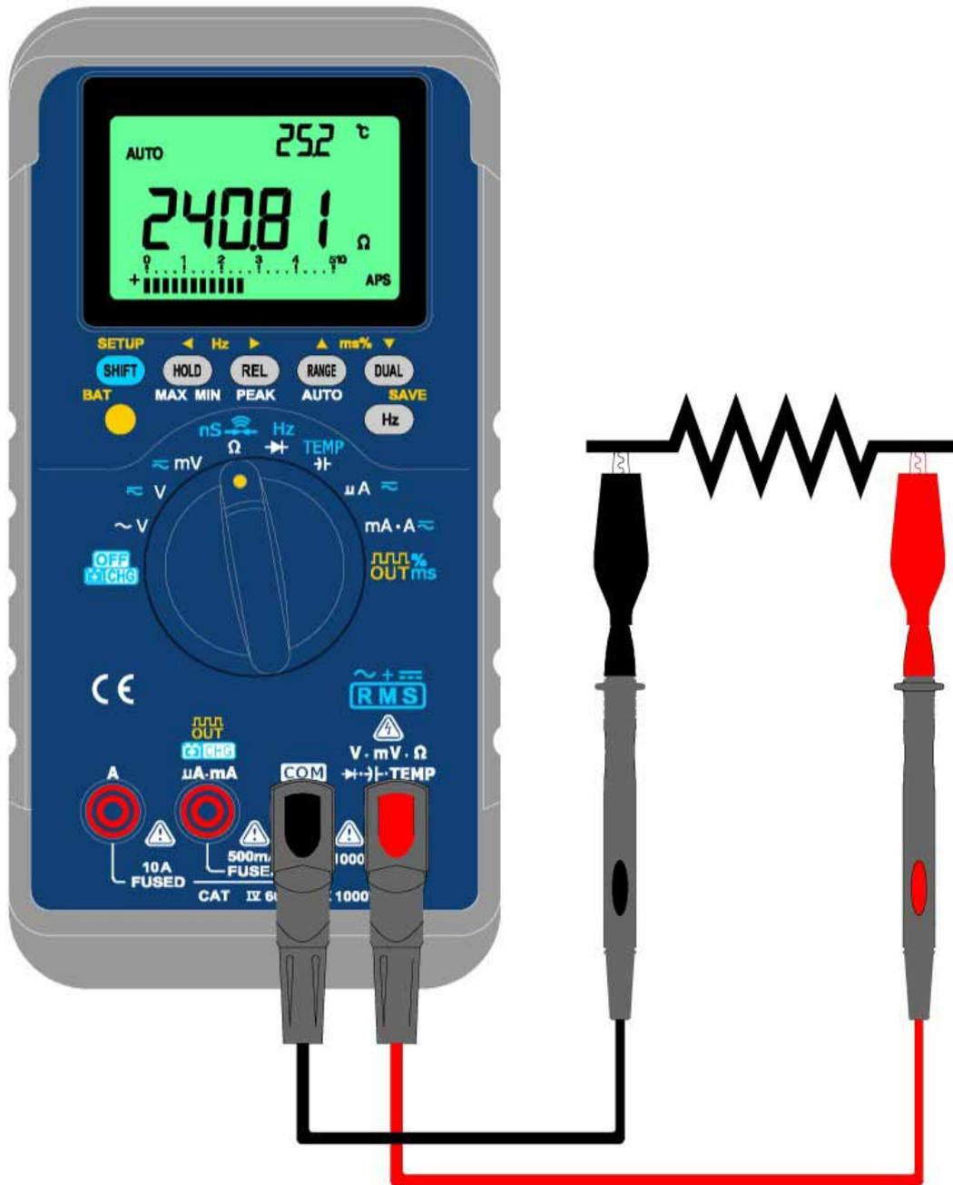
Figure- 50 Resistance measurement
