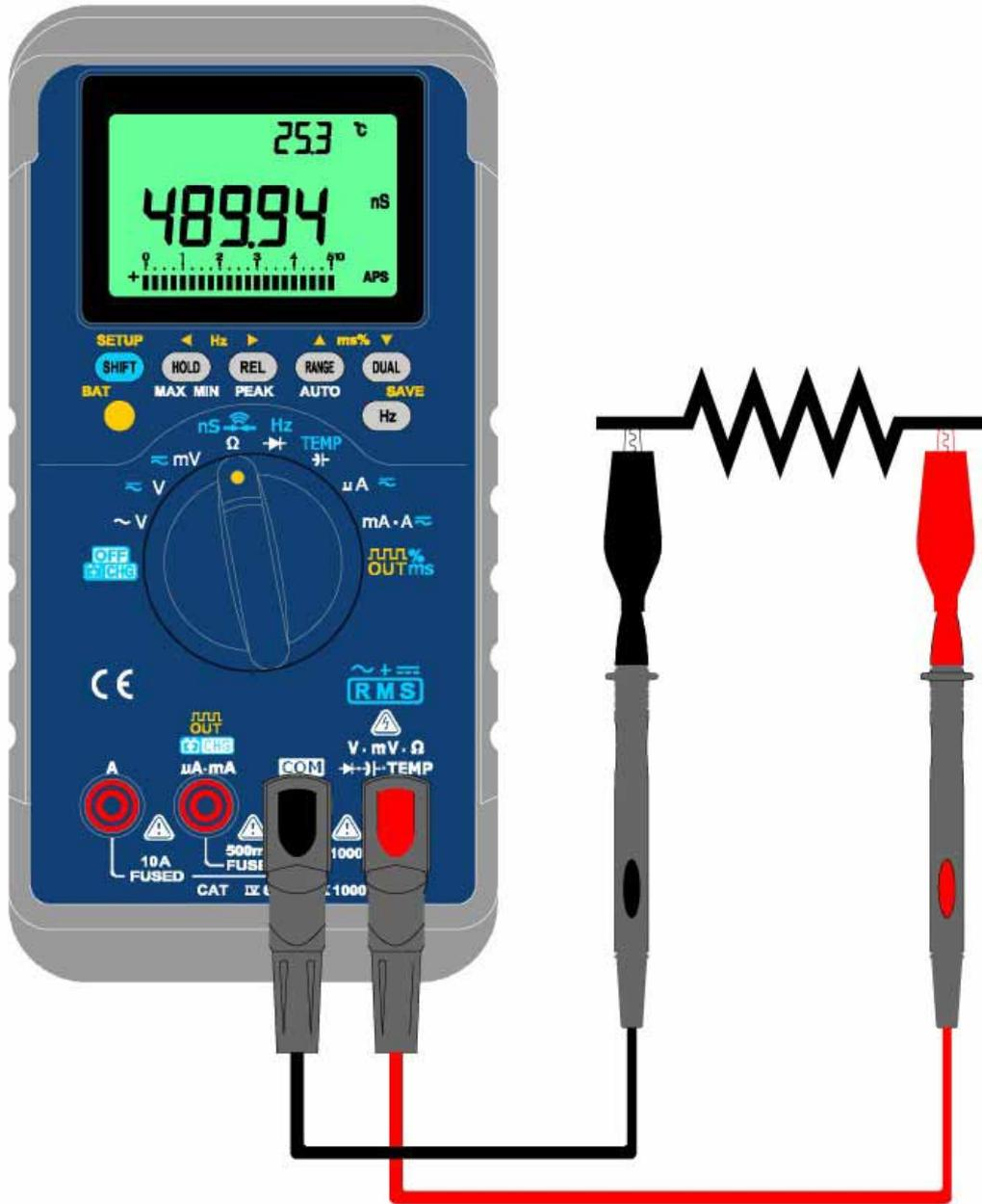
Figure- 51 Conductance measurement
