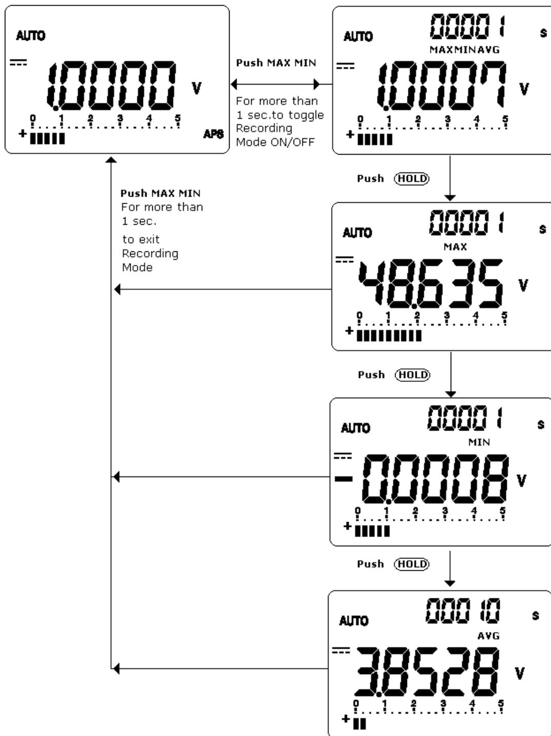
Figure- 29 Display of Dynamic Recording
