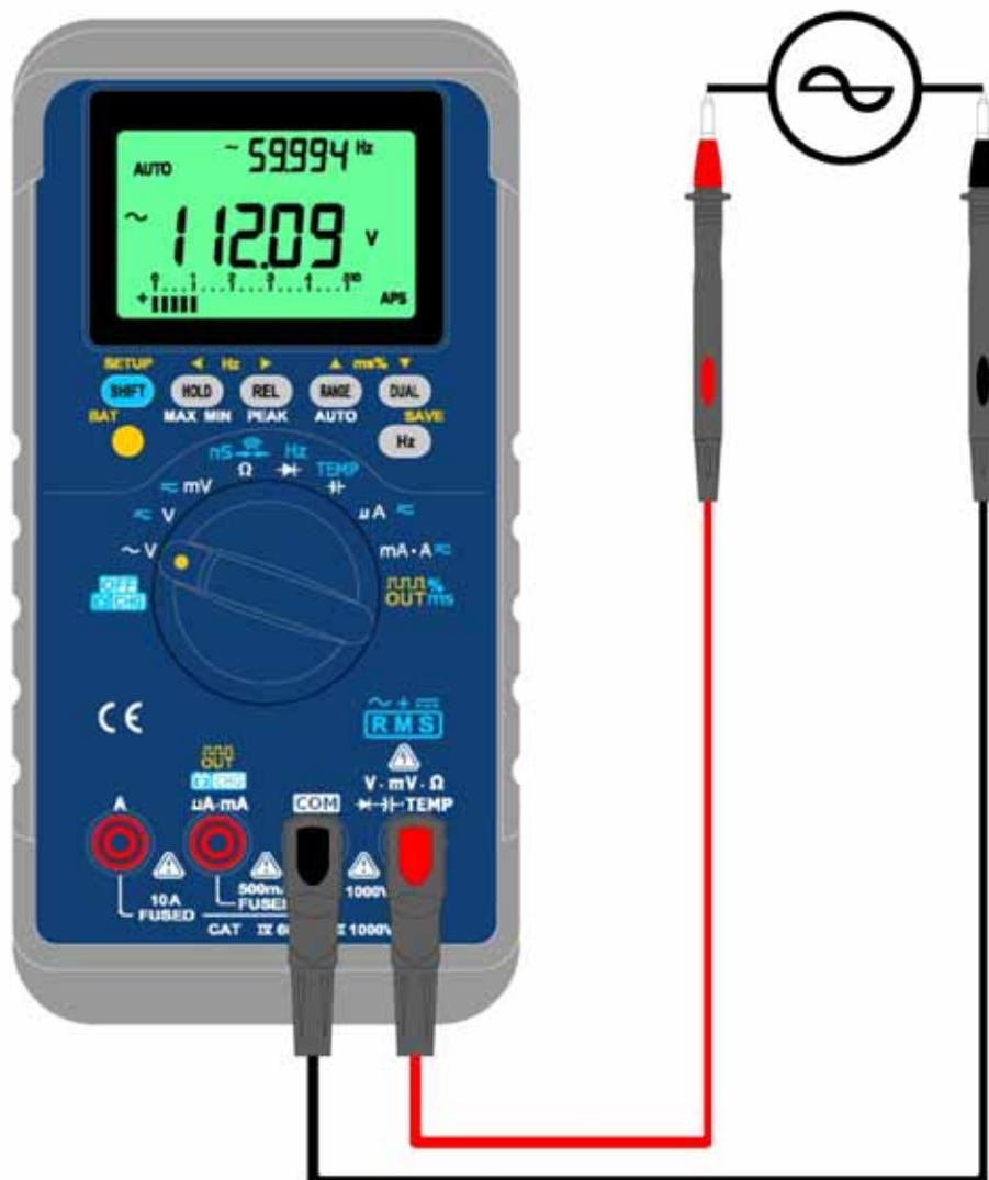
Figure- 1 Dual display for ACV/ Hz Measurement
