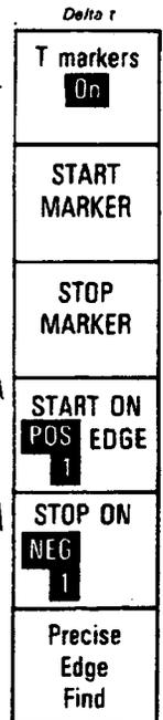
Connect the cal signal to Chan 1 and press the AUTO-SCALE control key. Select the delta t menu and turn the t markers on. Manually move the start marker so that it coincides with the first positive leading edge of the cal signal (Figure 6-6. This is one way of making a time interval measurement.
