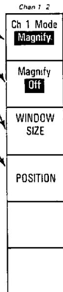
You would use the magnify function if you wanted to evaluate a small signal such as a reflection or overshoot that was present on large signal. Magnify can also be used to provide increased vertical sensitivity.
