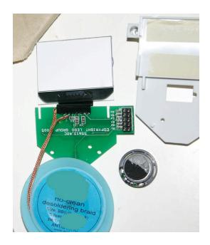
**LCD** glasses require an AC voltage to **polarize** the liquid media in the glass. And it uses a special scanning procedure to display dots. and as it uses high frequencies to do that, so any cold welding on the available capacitors on this PCB could affect the display.
