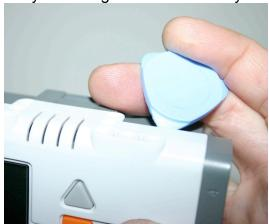
05- Use a hair blower to heat up the self dual side adhesive rear the LCD screen. And slowly... easy... carefully remove the LCD from the white plastic base form the lower corners. And Be Carefull not to touch the black flat to do that. As several companies mention that you shouldn't unplug electric cords from the wire! So please if you are not familiar with such thing, try it first in a damaged cheap Calculator.
