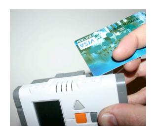
04- It's more professional to use special plastic tool to do that. You can find it in any electronic store such as mobile repair Stores. They are using it to dismantle tiny mobile plastic covers.
